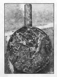
ABOVE: Rayo de la Muerte, a large, omnidirectional claymore-type mine with rebar fragments set in a matrix of beeswax.
